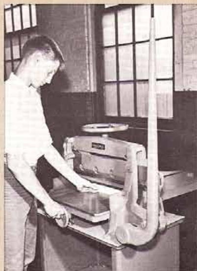
1. Place the paper stock on the table and move the back gage to the exact dimension for your cut.
