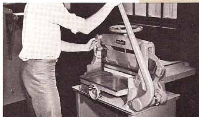
3. This is the two-handed safety control. Hold the safety handle with your left hand and start the knife bar down with your right hand. You have to keep holding the safety handle with your left hand until after the knife bar clears the safety pin.
